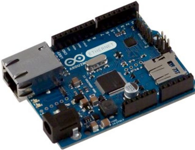
The Arduino Ethernet board is a 2-in-1 board that combines an Arduino micro-controller board and an Ethernet shield, all on a single board. Alternatively, you could use a separate Arduino Uno board combined with an Arduino Ethernet shield.
