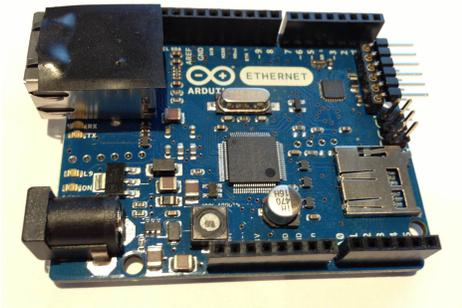
The DFRobot Relay Shield design has pins underneath it, that, if not properly protected, could produce a short-circuit when connected onto the Arduino Ethernet board.
